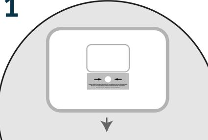
Press the sensor indicated by the arrows for 5 seconds to start the unit.
