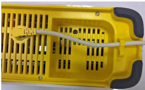
Figure 8: Power Cable Connected to Sprint Magic Box Gold
